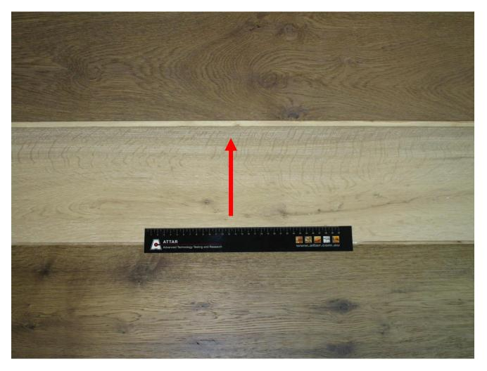
**Figure 1:** Prestige Engineered Oak 190mm & 220mm stair tread and nosing. Arrow indicates direction of testing.
