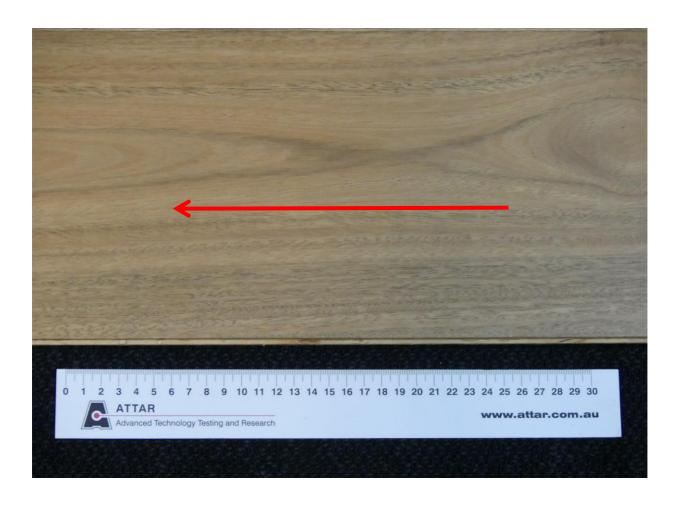
Figure 1: Eng Aust. Species smooth matte plank Arrow indicates direction of testing
